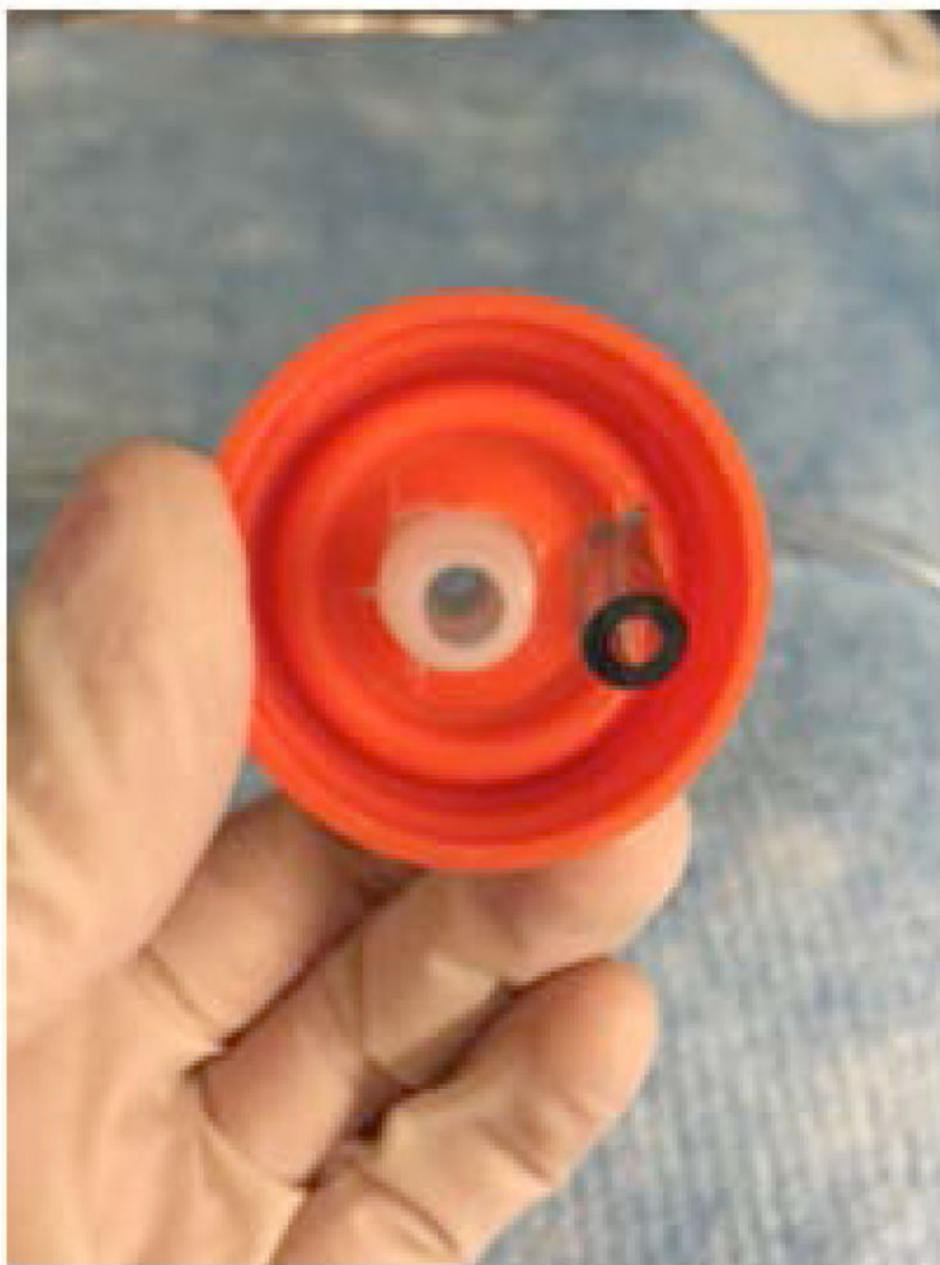
Figure 3. Bottom view of cap showing quick-connect coupler and thin tubing inserted.
