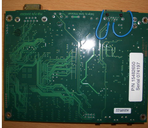
Figure A.6: The wires soldered to the ethernet jack pins on the bottom of the Soekris net4826 board.
