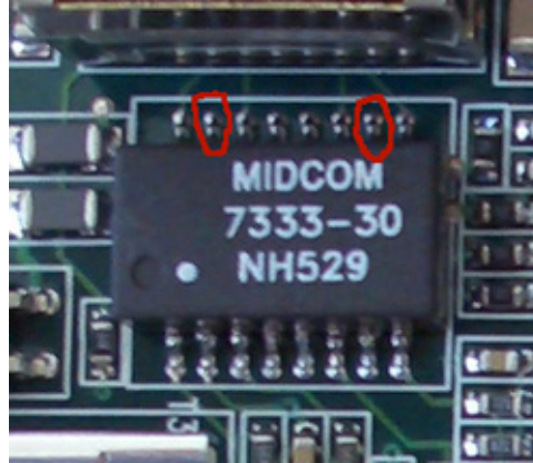
Figure A.3: The location of the center tap pins for the ethernet isolation transformer on the Soekris net4826 board. Each of the two pins is circled.
