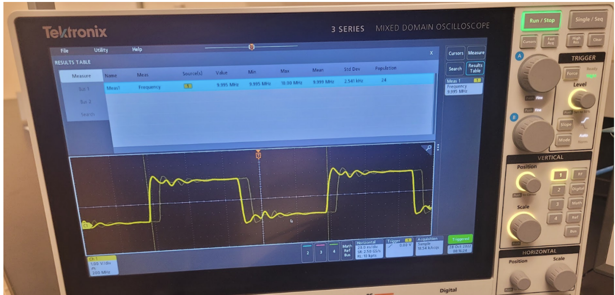
Figure 3.8: Bench measurement of the 10 MHz tile clock signal, with mean, maximum and other information provided by the oscilloscope.
