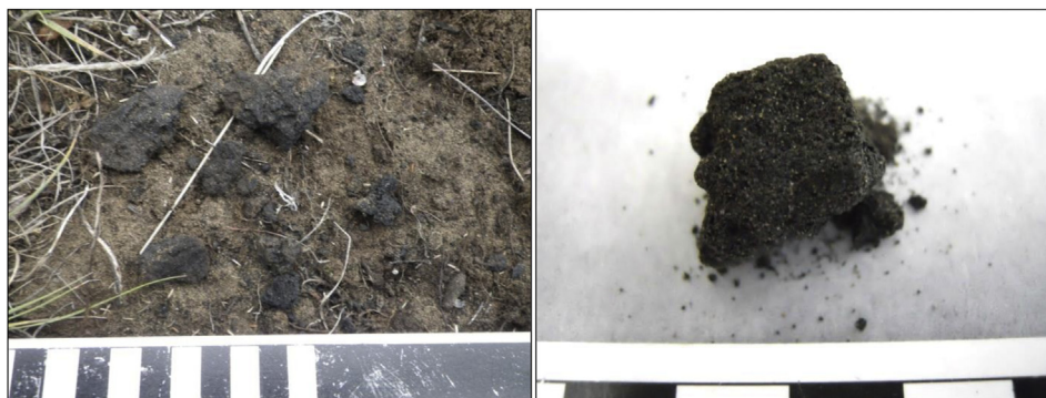
Fig. 2. Images of cemented sand from KTZ-325: in the field (left) and in the lab (right) (scale is in centimeters).
