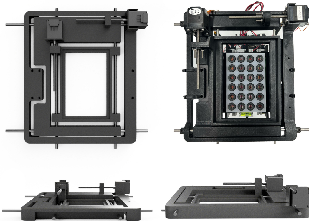
Figure 3.10: XY Plate Translation Stage XY positioning stage allows the position of the culture plate to be controlled so that areas of interest can be brought into the cameras field of view
