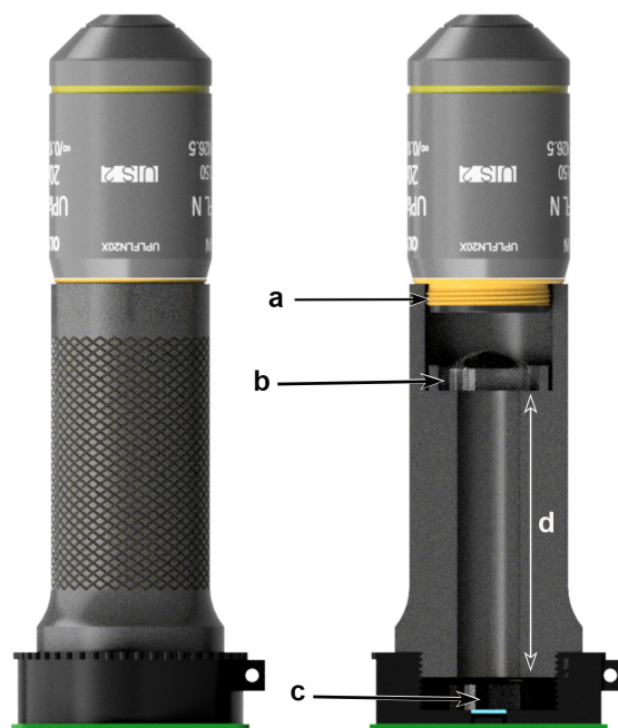
Figure 3.6: Fluorescence unit optics , a : standard RMS thread allows compatibility with many different off-the-shelf microscope objectives, b : tube lens allows for shorter optical tube, c : fluorescence emission filter sits atop sensor within the optical tube, d : tube lens position calculated based on our camera system as shown in appendix A.1
