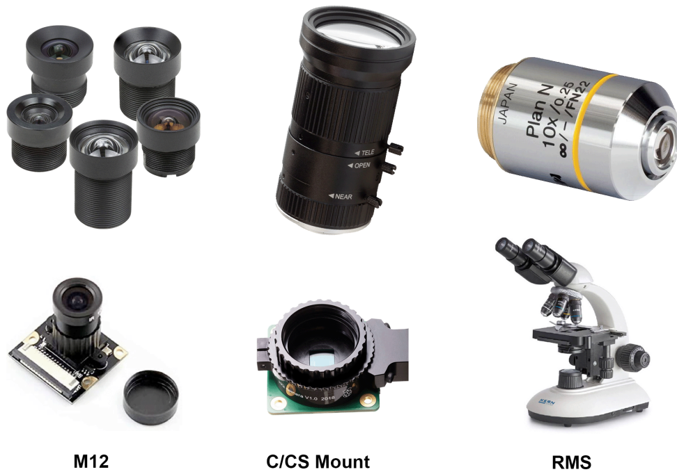
Figure 3.3: Options for Lens Optics M12 lenses are compact and low profile, C/CS mount optics are compatible with larger image sensors, RMS microscope optics have high zoom but require complex mounting systems.
