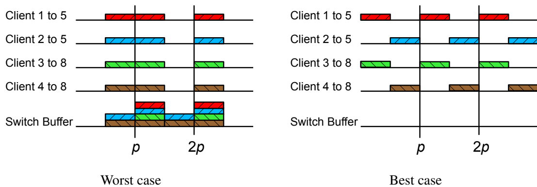
Figure 1.4: Time-series plot of a switch buffer with and without congestion
