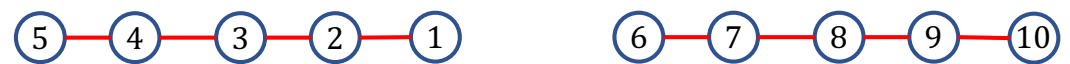
Figure 6. Graph connection topology of Formation-1. Mobile agents are connected only with their neighboring agents. The red line shows the connection between the agents.
