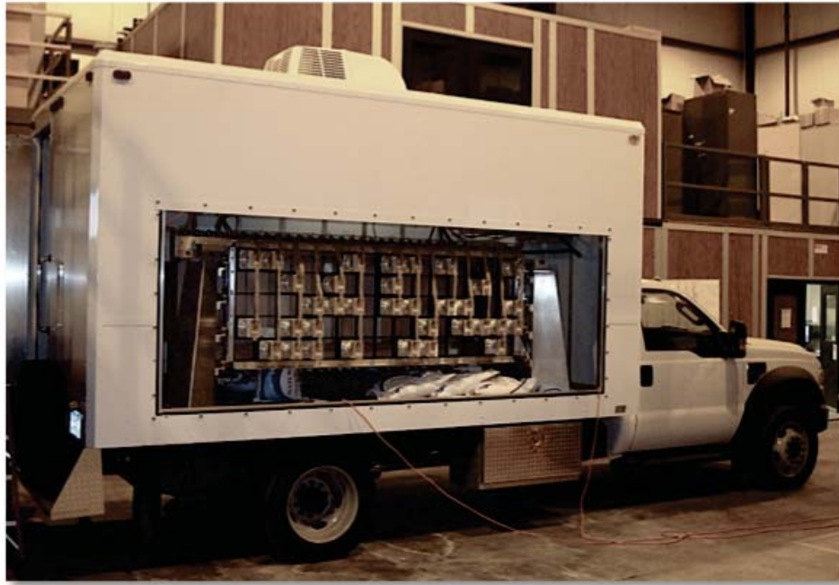
Figure 1.3: The TMI prototype system with the side panel removed to allow visibility into the detector system.
