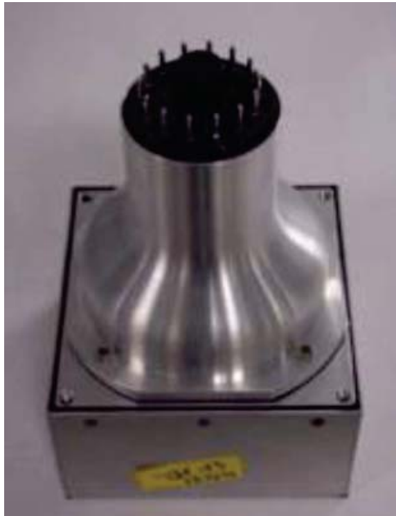
Figure 3.5: CA detector element assembly with photomultiplier tube attached.
