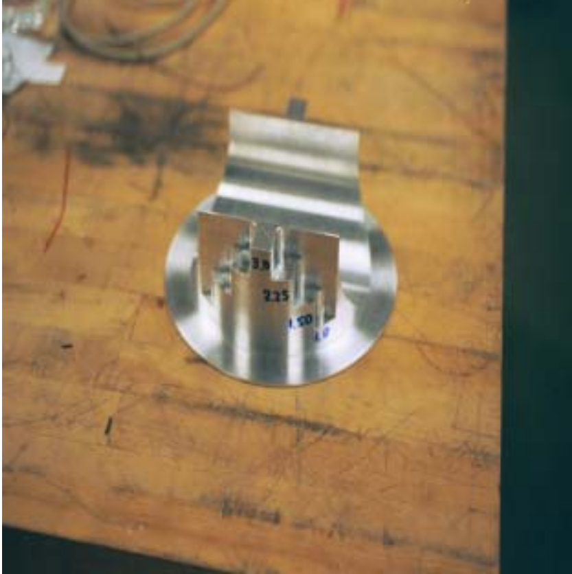
Figure 3. Aluminum x-ray compensator mounted in the front of the image intensifier. The curvature flattens the image intensity to account for the circular core cross section. The outer machined flats provide for calibration and normalization of x-ray beam intensity.
