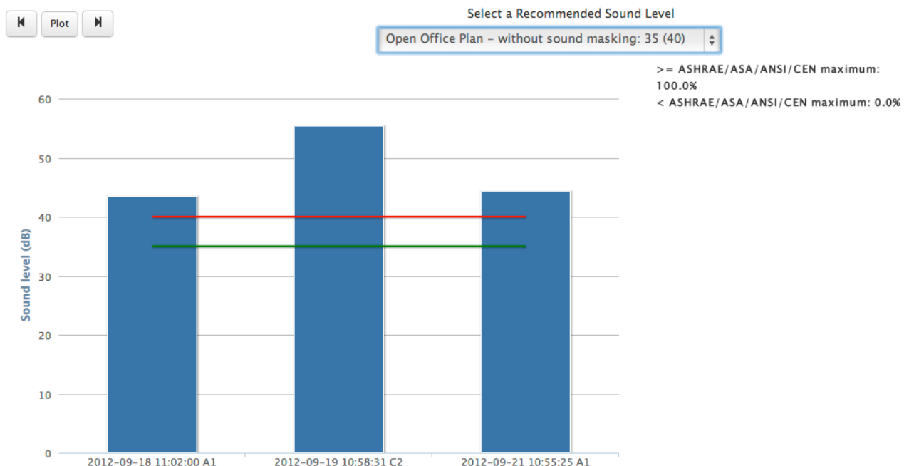
Figure 35: Acoustics example of whole-period analysis column chart
