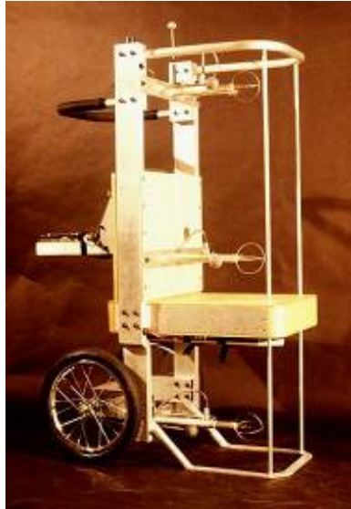
Figure 5: Instrumented chair-like cart (Benton, Bauman, & Fountain, 1990)
