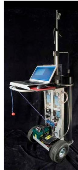
Figure 7: UFAD commissioning cart (Webster, Bauman, & Anwar, 2007)
