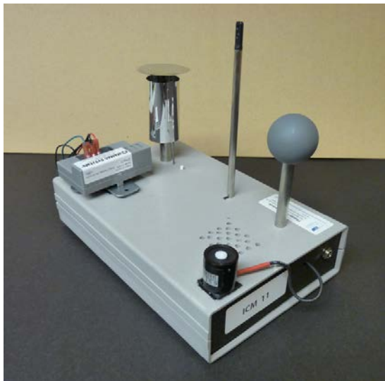
Figure 10: ICM device with CO 2 , illuminance, globe, air velocity, dry bulb temperature, and relative humidity
