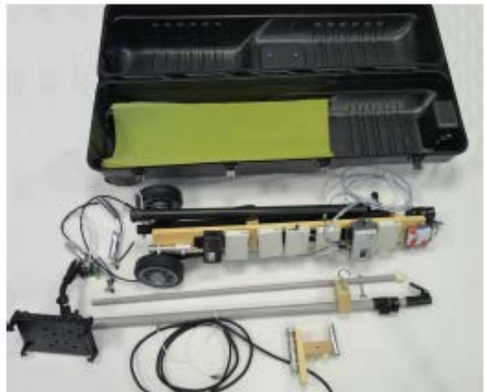
Figure 13: PUCC disassembled and ready for transport in golf bag carrier
