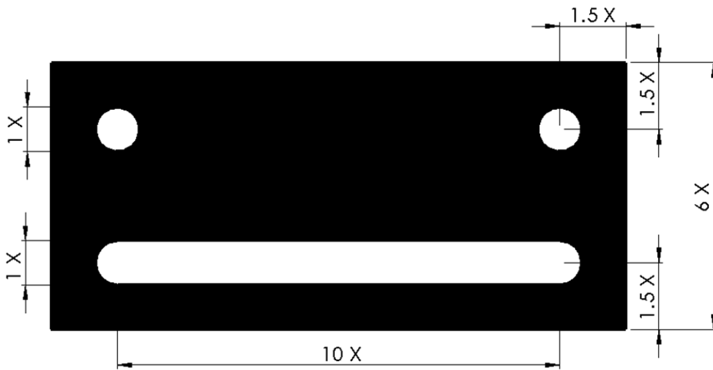
Figure 2-3: 2-Layer Device Dimensions. The 2-layer devices are all similar in dimensions. The lower channel is 10 times as long as the channel is wide and all borders are designed to be as thick as the channel is wide after melting.
