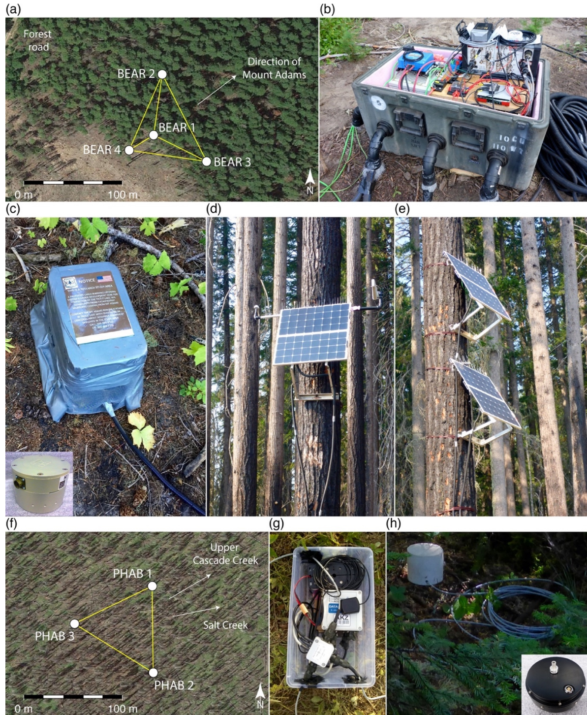
Figure S1. (a) Geometry of the BEAR station (4-element infrasound array) with PMCC subarrays shown in yellow. (b) BEAR Pelican-Hardigg vault containing the data logger, cell modem, solar controller, fuses, and lightning arrestors. (c) Hyperion IFS-3111 infrasound sensors (inset) are covered to provide basic protection from animals and snow accumulation. (d, e) Six 100 W solar panels, GPS and cell antennae mounted in trees on edge of clear-cut. (f) Geometry of PHAB station (3-element array), which has no subarrays. (g) PHAB/CHIP/RAIN central recording hub, including digitizer, GPS, power supply and breakout box to connect to the infrasound sensors. (h) Chaparral Model 60-UHP infrasound sensor (inset) inside foam wind filter, as used at PHAB/CHIP/RAIN.
