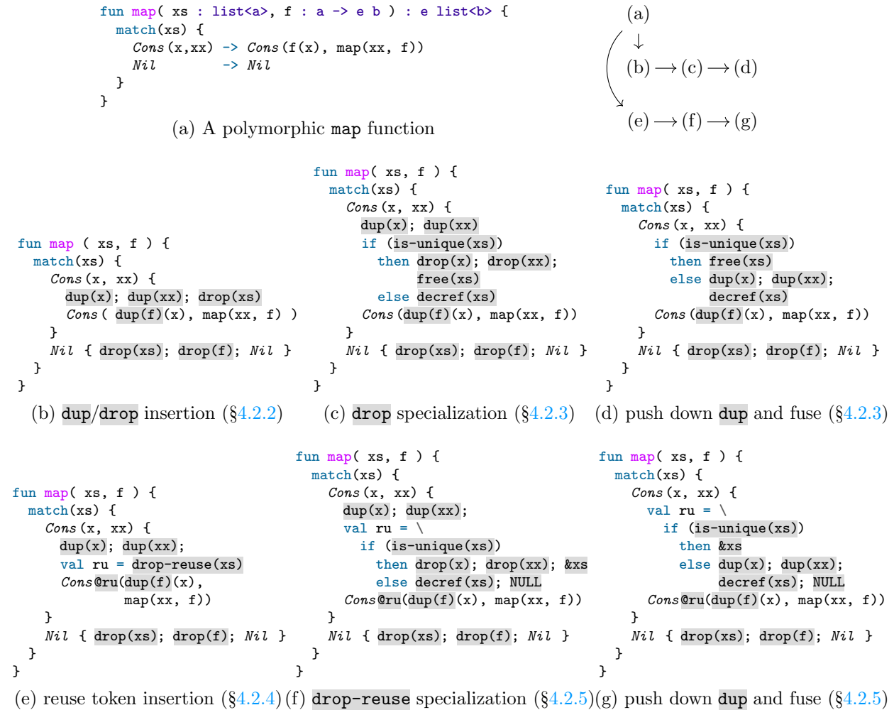
Figure 4.1: Drop specialization and reuse analysis for map.
