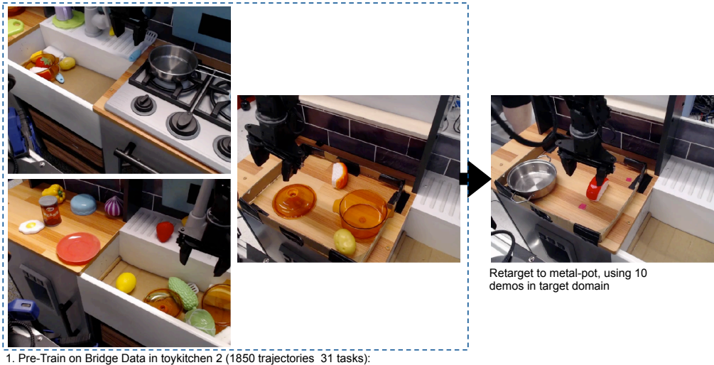
Figure D.5: Illustration of pre-training data and finetuning data used for Scenario 1: re-targeting the put sushi in metal-pot behavior to put the object in the metal pot instead of the orange transparent pot.
