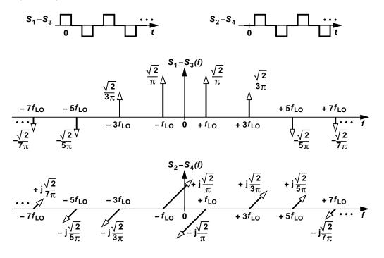
Figure 4.7:  $(S_1 - S_3)$  and  $(S_2 - S_4)$  in time and frequency domains.
