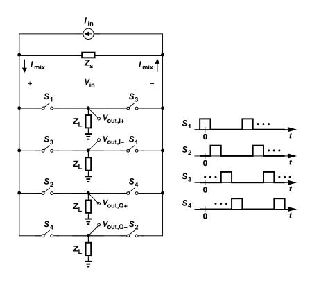
Figure 4.6: Current-driven passive mixer and LO waveforms.
