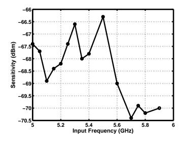
Figure 4.19: Measured sensitivity.
