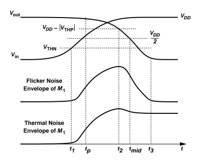
Figure 2.5: Detailed view of thermal and flicker noise envelopes during input and output transitions.
