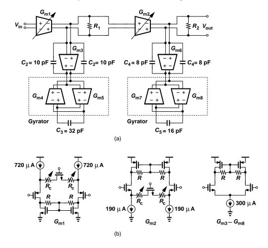
Figure 4.14: (a) Fourth-order elliptic low-pass filter, and (b)  $G_m$  implementations.
