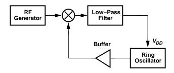
Figure 3.11: Phase-locking of the ring oscillators for phase noise measurements.
