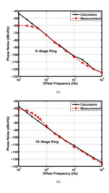
Figure 3.12: Measured phase noise of ring oscillators and the calculated phase noise using the measured phase noise of delay line for (a) 9-stage, and (b) 19-stage rings.
