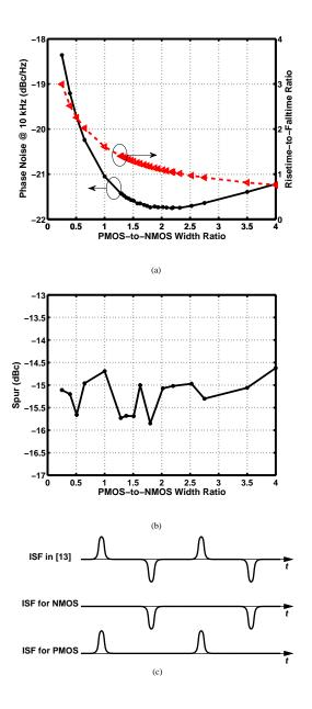
Figure 3.5: (a) Phase noise and risetime-to-falltime ratio versus the PMOS-to-N-MOS width ratio of a 9-stage 2.4-GHz ring oscillator, (b) spur power when a small sinusoidal voltage source is put in series with the gate of one NMOS transistor in the ring, and (c) ISF reported in [13] and uncorrelated ISF's for NMOS and PMOS devices.
