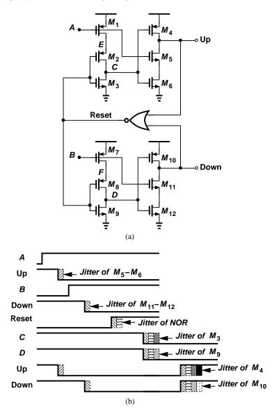
Figure 2.10: (a) TSPC PFD, and (b) jitter contributions to the outputs.
