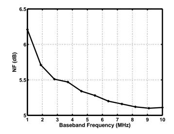
Figure 4.16: Measured noise figure.
