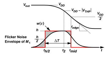
Figure 2.6: Rectangular approximation of noise envelope.
