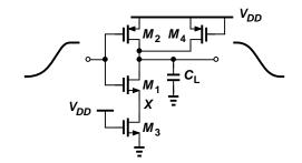
Figure 2.8: NAND gate with one input changing.
