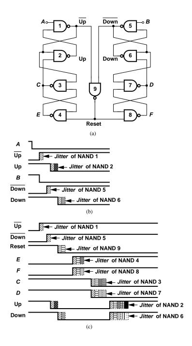
Figure 2.9: (a) NAND-based PFD, (b) jitter contributions to falling edges of outputs, and (c) jitter contributions to rising edges of outputs.
