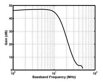
Figure 4.21: Measured receiver transfer function.
