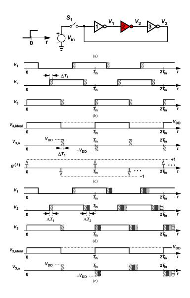
Figure 3.2: (a) Three-stage ring oscillator retimed at t = 0 with only one noisy inverter, (b) jitter on all edges due to a single jitter event on  $V_2$ , (c) decomposition of  $V_3$  in (b) to an ideal noiseless square wave and a noise waveform, with g(t)serving as a "carrier," (d) jitter on edges when inverter #2 adds jitter on every transition, (e) decomposition of  $V_3$  in (d) to an ideal noiseless square wave and a noise waveform.
