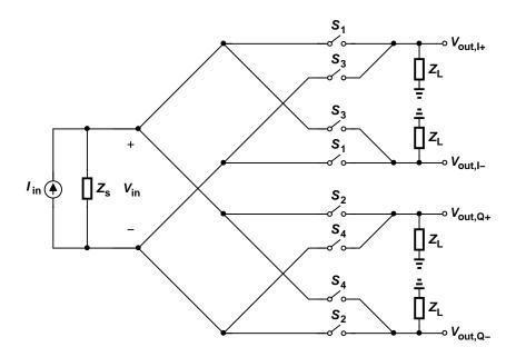
Figure 4.5: Current-driven passive mixer.
