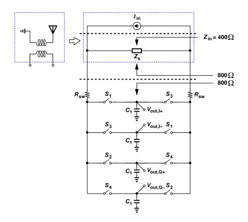
Figure 4.12: Transformer-mixer interface.
