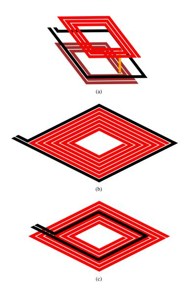
Figure 4.2: Various transformer topologies.
