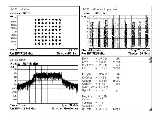
Figure 4.17: Measured EVM at  $P_{in} = -65$  dBm.
