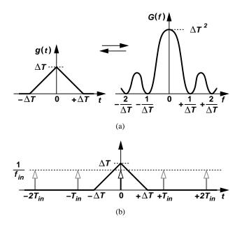
Figure 2.19: Inverse Fourier transform of (a)  $sinc^2$  function, and (b) shifted  $sinc^2$  functions.
