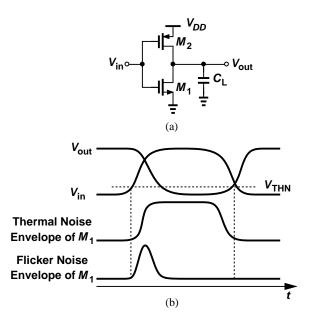
Figure 2.4: (a) CMOS inverter, and (b) thermal and flicker noise envelopes of  $M_1$ .
