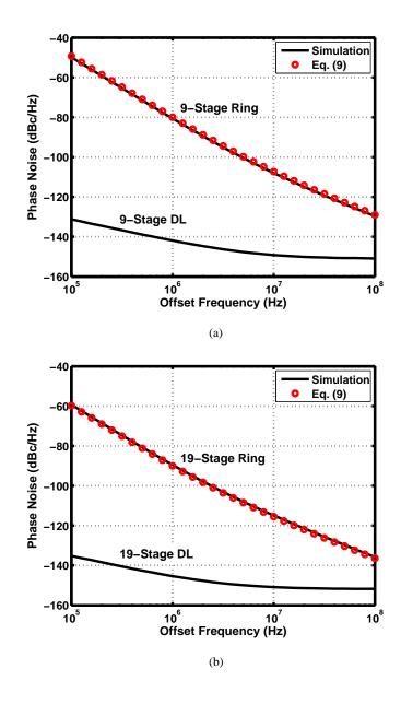
Figure 3.6: Simulated phase noise of delay lines and ring oscillators as well as calculated phase noise of the ring oscillator using the phase noise of the delay line for (a) 9-stage, and (b) 19-stage configurations.
