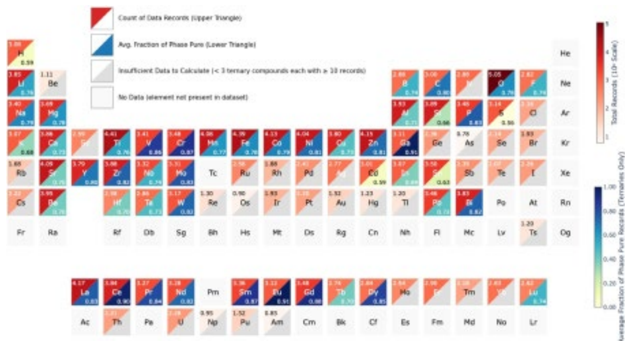
Fig. 2 Target materials elemental frequency and phase purity trends. Upper left triangle: total data records ( 10^x scale). Lower right triangle: average fraction of phase-pure records calculated from ternary compounds. Elements with less than three ternary compounds with at least ten data records each are excluded from phase purity analysis (dark gray). The figure includes 117,831 of the 148,024 records (79.6%). The remainder are excluded because the target formula could not be normalized by text2chem or parsed by pymatgen.
