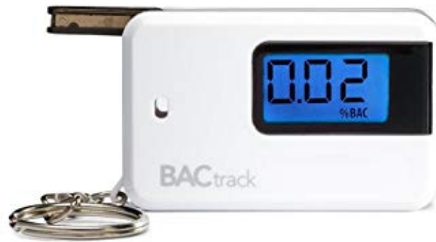
Figure 3. “BACtrack Go” portable alcohol breathalyzer used in the current study. This breathalyzer includes a keychain ring and a fold-out mouthpiece for portability.
