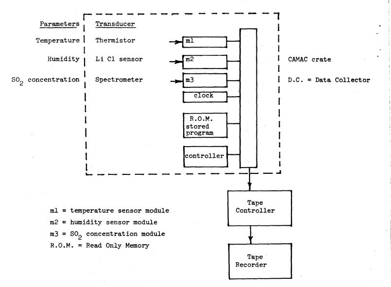
Block diagram of a small portable environmental sensing station.
