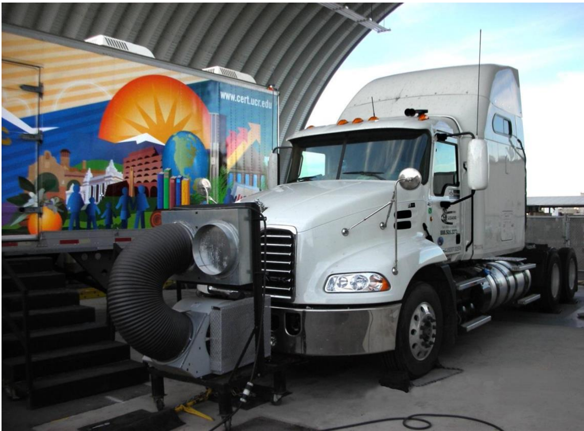
Figure 20. UCR's Heavy-Duty Chassis Dynamometer test facility
