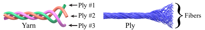
Figure 3: Fabric structure: a yarn normally consists of multiple sub-stands called plies. Each ply in turn contains tens to hundreds of micron-diameter fibers.
