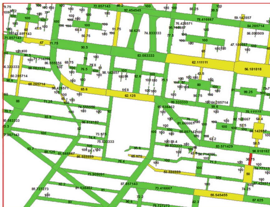
Fig. 14 PCIs of a considered part of the studied pavement network with proposed methods at project level (PSO-GA)
