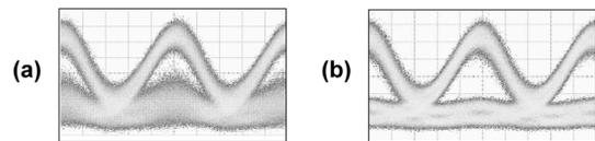
Fig. 3 Eye diagrams for 16 time-slotted users taken at the output of (a) the NOLM and (b) the output of the thresholder.
