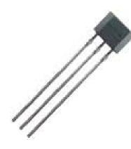
The Hall Effect sensor that our gaussmeter is using is called the Honeywell SS49E Hall Effect Sensor. This hall effect sensor outputs an analog voltage that depends on the sensed magnetic field intensity that is perpendicular to the sensor face. The sensor circuit uses difference op amps for better precision.
