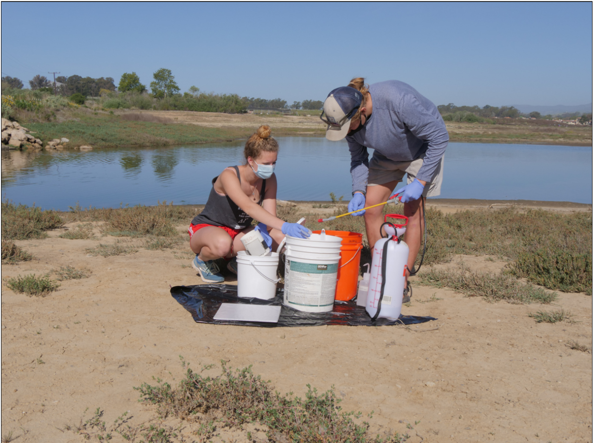
Students Bailey Kimery and Cole Diemer cleaning E-DNA sampling materials with DI water to prevent contamination.
