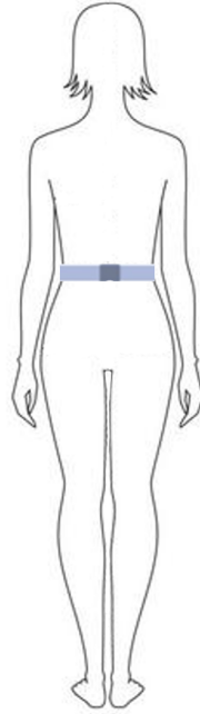
Figure 4.2: Position of an APDM Opal inertial sensor attached to the lumbar region using a stretchable belt. The sensor was placed on the lower back of the subject. Accelerometer, gyroscope, and magnetometer data was collected as subjects walked back and forth for 2 minute (as part of the UPDRS Part III test) while wearing this sensor.
