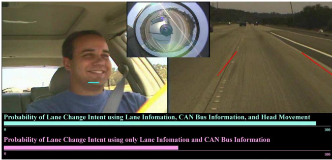
Fig. 11. Example of detection of lane-change intent. The top bar shows the estimated probability of lane change using all the three sources, whereas the bottom bar shows the probability using only lane tracking and CAN bus data. The lane change is detected earlier when head-motion information is used.
