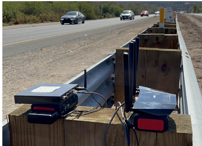
Figure 5.6: An RSU connected to a cellular router on the highway.
