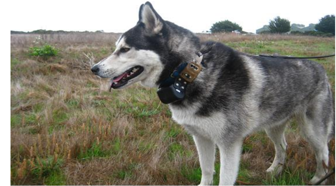
Fig. 4 Siberian husky wearing accelerometer collar during calibration trial
