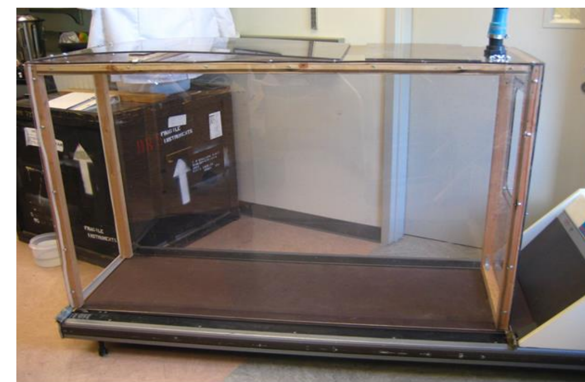
Fig. 7 Metabolic chamber sitting above treadmill belt
