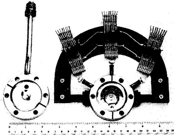
Fig. 6a. Photograph of the chamber sketched in Fig. 5. Flange at left shows vacuum and fill pipe. Flange at right shows ceramic disk and three 8-conductor feed-throughs. The printed circuit boards contain capacitors and resistors to allow the anode wires and charge amplifiers to operate at different potentials.
