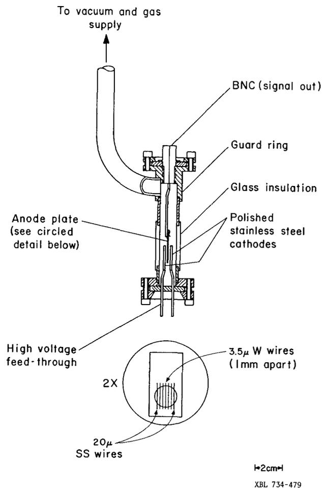
Fig. 4. Multi-wire test chamber. Cathodes are polished stainless steel plates, one containing an  $^{241}\text{Am}$  source. Anode is a stainless steel plate with  $3.5\text{-}\mu$ -diameter wires stretched across a hole.
