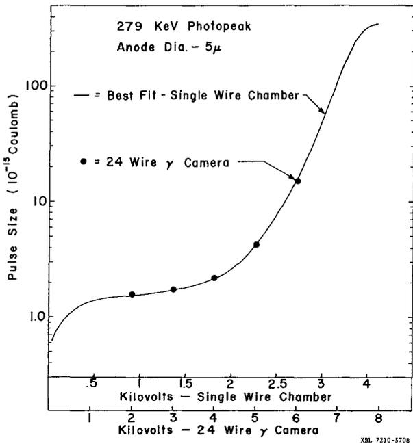
Fig. 2. Pulse height vs voltage for 5- $\mu$  wire. Solid curve: data from single-wire chamber; dots: data from 24-wire proportional chamber. Due to differences in geometry, the voltage scales differ by a factor of 2.2.
