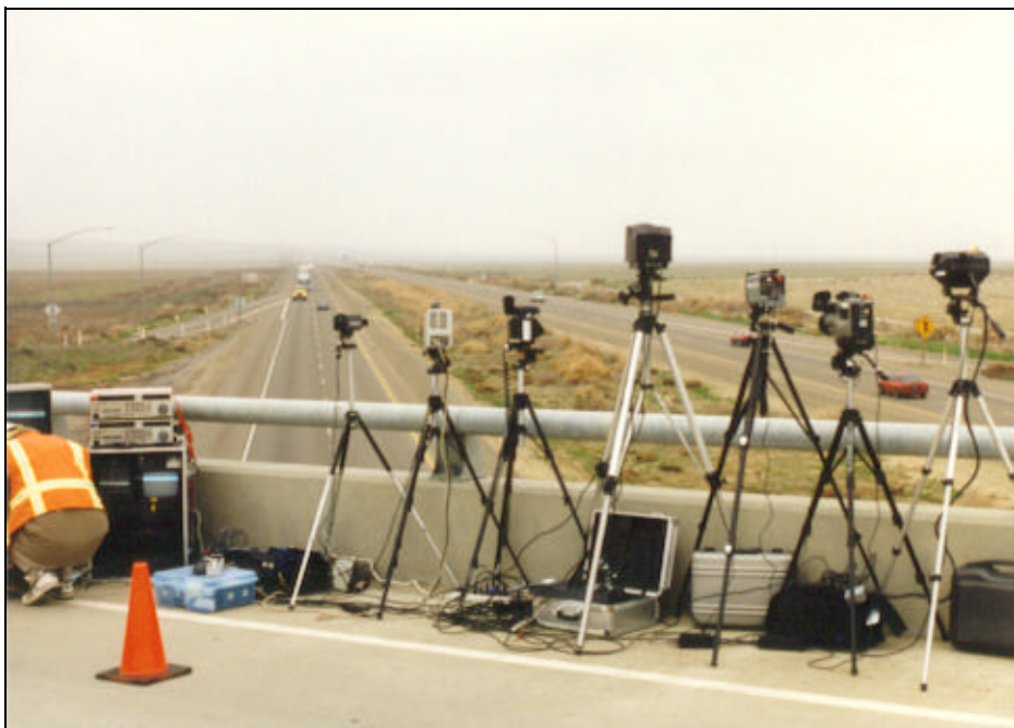
Figure 13.4 Typical Simultaneous Camera Test Setup, Interstate Hwy 5, near Manteca.
