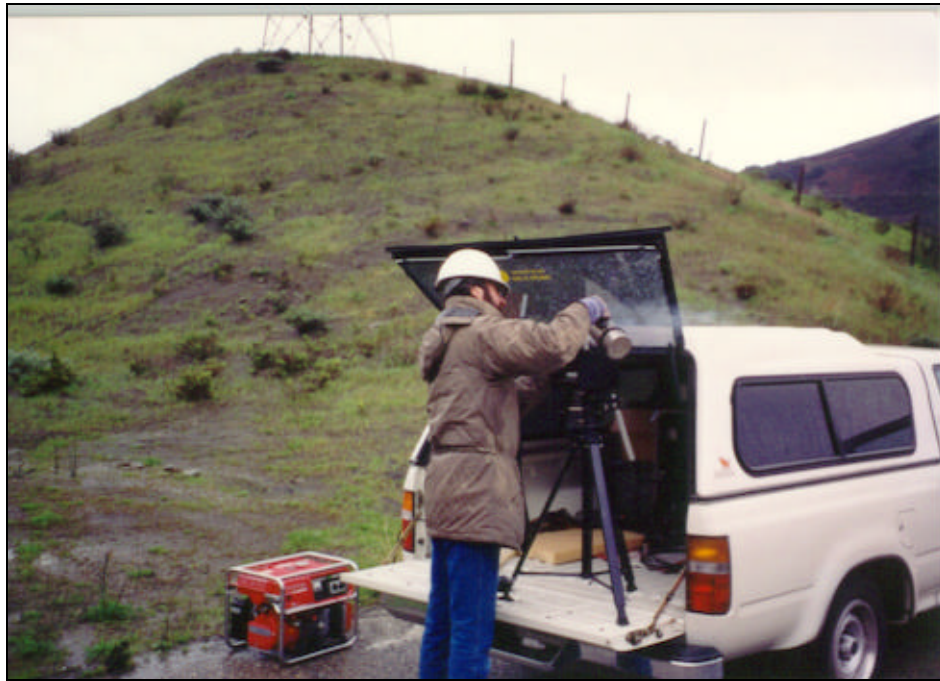
Figure 13.10 Filling the Inframetrics 610 Dual-band IR camera with Liquid Nitrogen.
