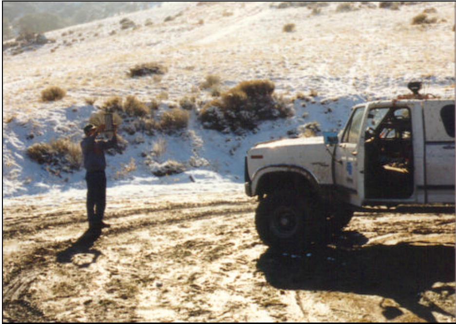
Figure 13.6 Resolution Testing Pyroelectric Infrared Camera Under Snow-glare Conditions.
