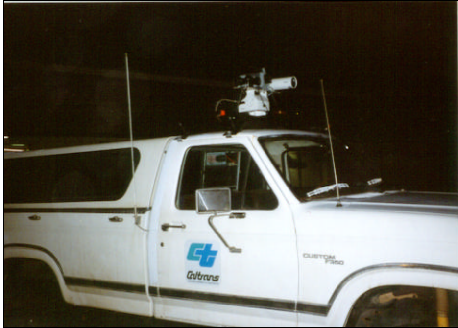
Figure 13.2a Exterior View of Mobile Data Collection and Tow Vehicle.
