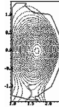
Fig.III.7.2.1 A loss orbit near X-point
