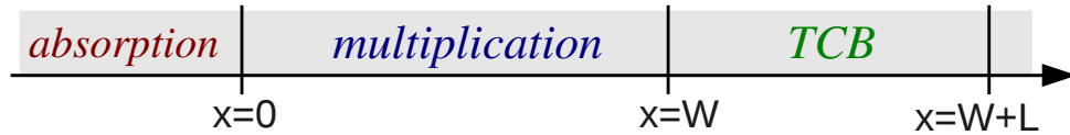
Figure 2.2: Regions of interest in the self-quenching SPAD model, with a valence band barrier for holes at x = W .
