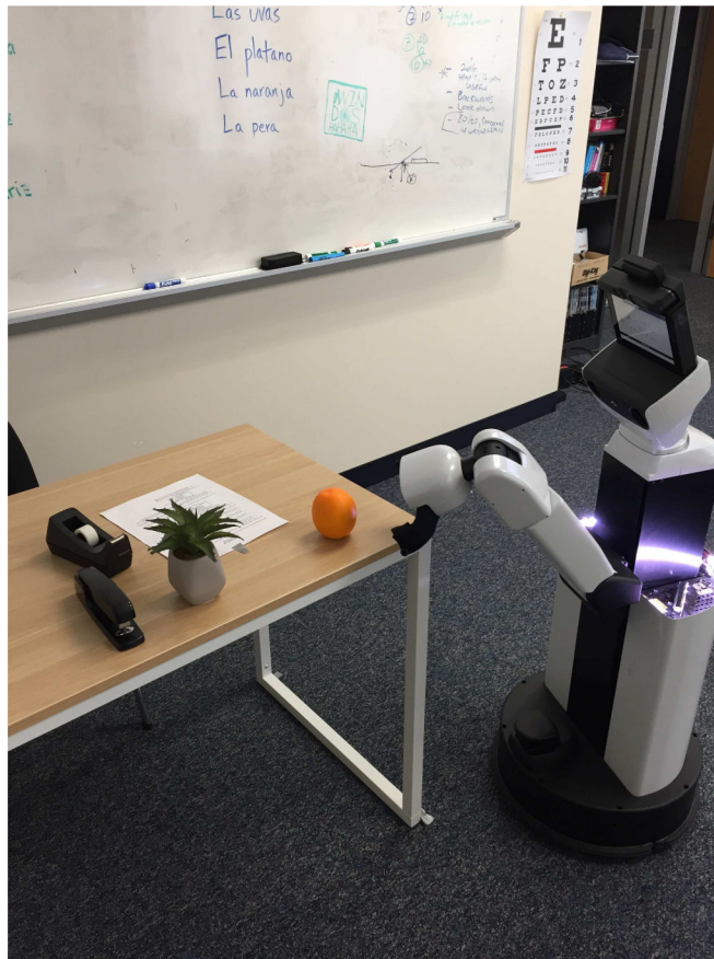
Fig. 5. The schema network from [31], [68] was implemented on the Toyota Human Support Robot (HSR). The HSR retrieved objects in a breakroom and a classroom schema. Search times decreased as the HSR learned which items belong to each schema.
