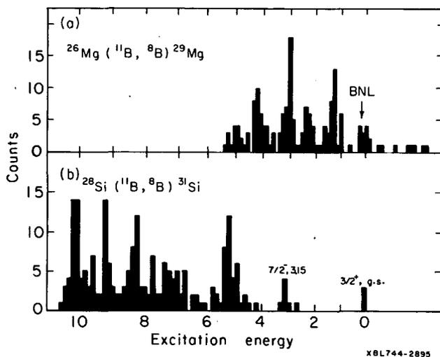
Fig. 10.  $^8\text{Be}$  spectra from  $^{26}\text{Mg}(^{11}\text{B}, ^8\text{B})^{29}\text{Mg}$  and  $^{28}\text{Si}(^{11}\text{B}, ^8\text{B})^{31}\text{Si}$  at  $E = 86$  MeV (lab) and  $11^\circ$  (lab).
