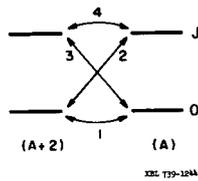
Fig. 4. Direct and indirect routes in two-neutron pick-up and stripping. In stripping to state  $J$ , route 3 is direct and in pick-up 2 is direct.
