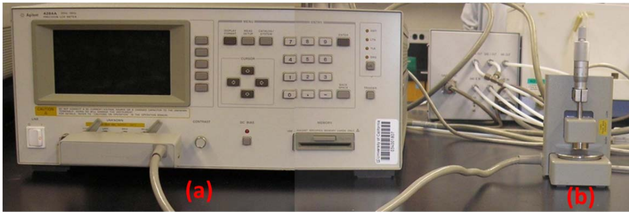
Figure 34: Agilent Technologies 4284A Impedance Analyzer (a) and 16451B Solid Dielectric Test Fixture (b)
