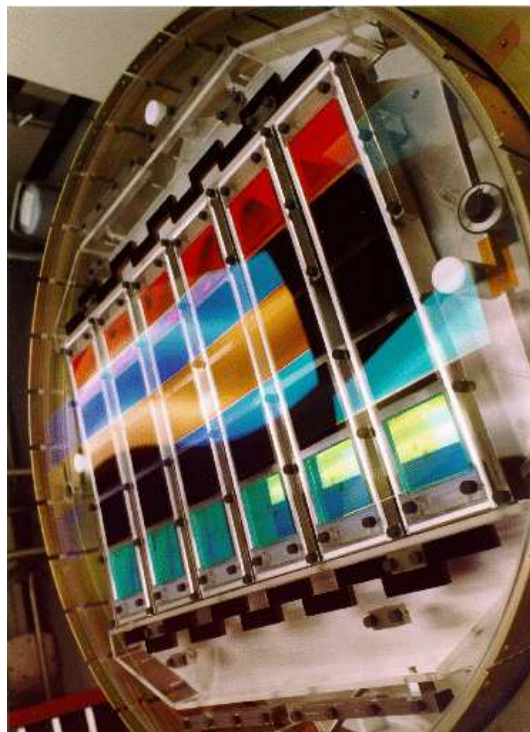
Figure 1.4: Faceplate of the CCDs on the main imaging camera of the Sloan Digital Sky Survey (SDSS) telescope. Image Credit: SDSS.
