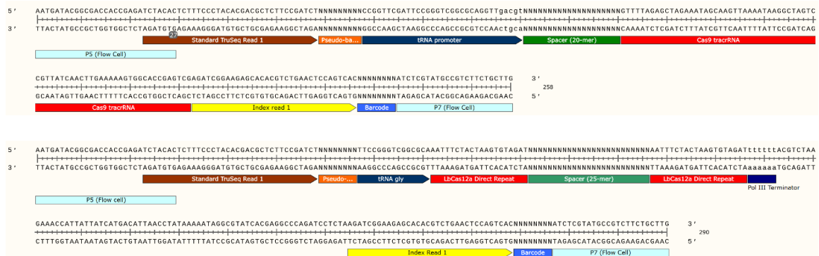
Figure S4.8. Schematic and sequence information of Cas9 (top) and Cas12a (bottom) amplicons for NGS. Amplicons contain (i) P5 and P7 sequences (light blue) that are necessary for binding with the flow cell in Illumina sequencers, (ii) TruSeq adapter (brown) for binding of the sequencing primer, (iii) a portion of tRNA gly (black) expressing the sgRNA, (iv) Cas9 or Cas12 spacer (green) (v) Cas12a associated direct repeats or a portion of the Cas9 tracrRNA sequence (red), (vi) Universal 8 bp Illumina barcodes (blue), (vii) Index read 1 sequence for the binding of primers to sequence the Illumina barcodes, and (viii) 4-9 nt pseudo-barcodes (orange) at the 5' end between the TruSeq and tRNA gly which help demultiplex replicates that contain the same illumine barcode.
