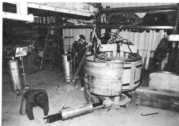
Figure 9. Nb_3Sn high field axicell coil cover installation.
