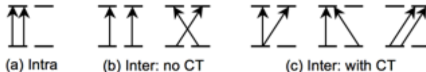
Figure 5.1: Classes of correlation amplitudes involving 2 fragments (each corresponding to a pair of levels in the diagram), which are separated to accomplish the EDA. (a) Intra-fragment correlations both occupied and virtual levels belong to a single fragment (the left one in the diagram). These contributions are included in isolated fragment energies (b) Inter-fragment correlations that do not involve charge transfer one correlated electron is associated with each fragment. These effects are included in addition to (a) in frozen and polarized energies (c) Inter-fragment correlations that are accompanied by charge transfer they included in the charge transfer energy in addition to (a) and (b).
