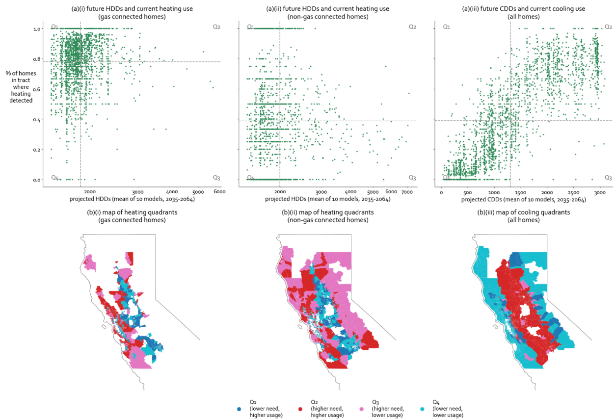
Figure 16 (a) projected heating/cooling needs and current heating/cooling usage with labeled quadrants and (b) map of quadrants for (i) heating use in gas-connected households, (ii) heating use in non-gas connected households, and (iii) cooling use in all households (note that figures (a)(i) and (a)(ii) use a log scale for the x-axis)
