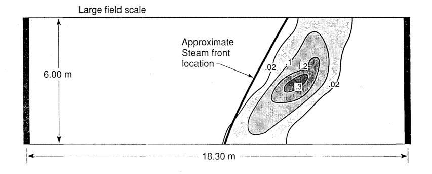
Figure 26. Separate phase xylene saturation distribution and steam front location after 106.5 days of steam injection.
