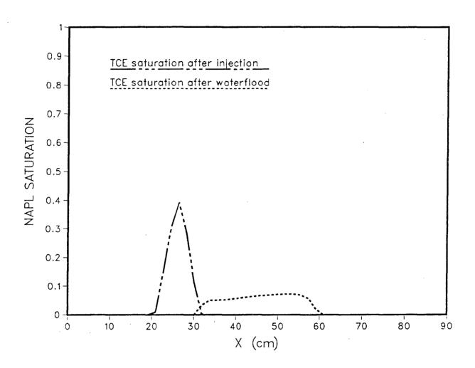
Figure 9. NAPL phase saturation distribution after trichloroethylene injection, and after waterflood.
