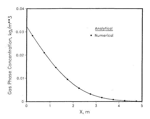
Figure 3. Comparison of STMVOC results with analytical solution of Baehr [1987] for transient diffusion with phase partitioning.
