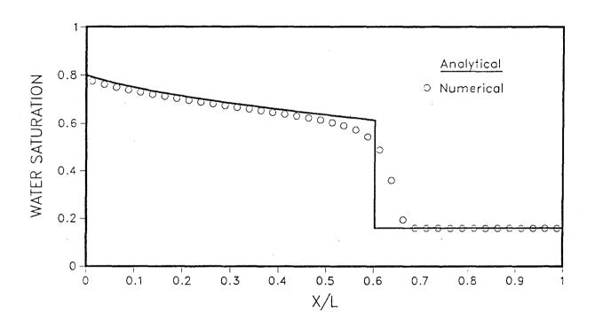
Figure 6. Comparison of STMVOC results with analytical solution for two phase flow.
