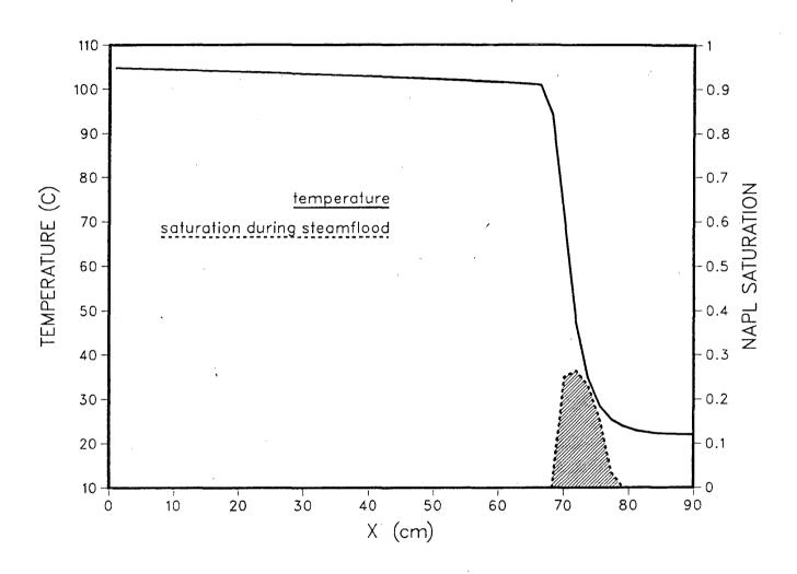
Figure 14. Calculated separate phase trichloroethylene distribution and temperature profile after 5000 s of steam injection.
