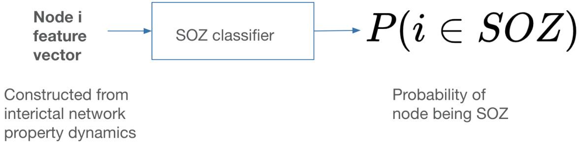
Figure 5.6: SOZ classifier setup: The SOZ classifier takes in as input a node feature constructed from the interictal network property dynamics and outputs a probability of the node being an SOZ
