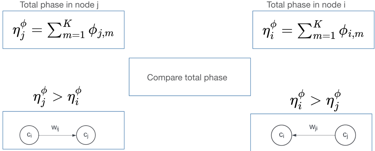
Figure 5.5: Edge directionality: If the total phase in channel j leads the total phase in channel i then we assign a directionality from i to j and if the total phase in channel j lags the total phase in channel i then we assign a directionality from j to i
