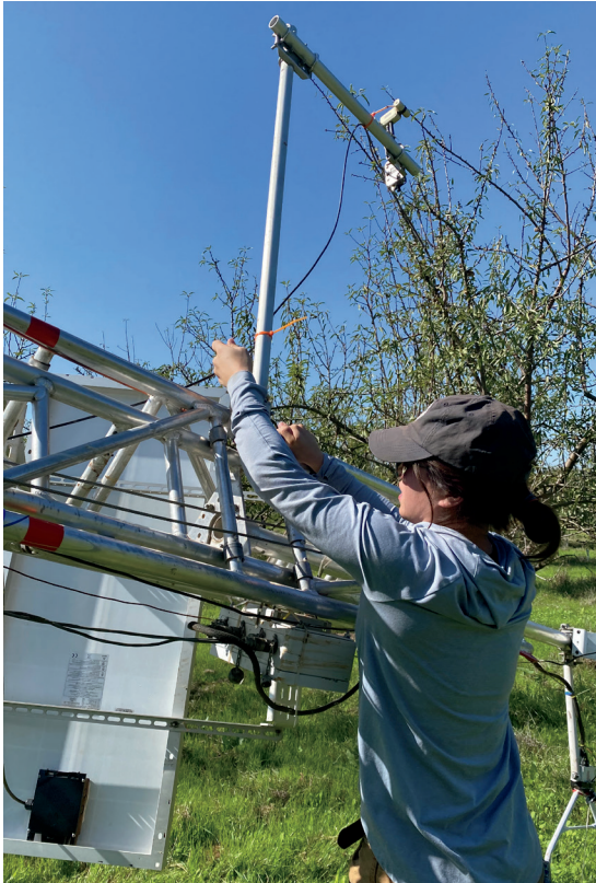
Author Margot Flynn repositions the net radiometer at MER (4) after routine cleaning. Photo: Olmo Guerrero-Medina.
