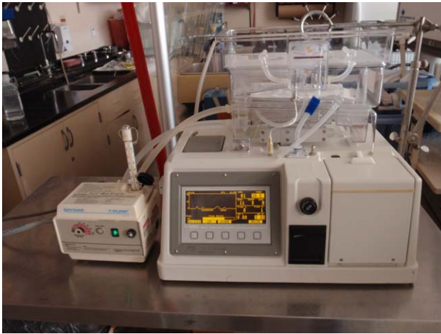
Fig. 2. RM3 pulsatile perfusion unit. The RM3 unit is displayed prior to priming with blood products. The circuit warmer is seen just to the left of the RM3, which maintains the perfusate at physiological temperatures. [Color figure can be viewed in the online issue, which is available at www.laryngoscope.com .]
