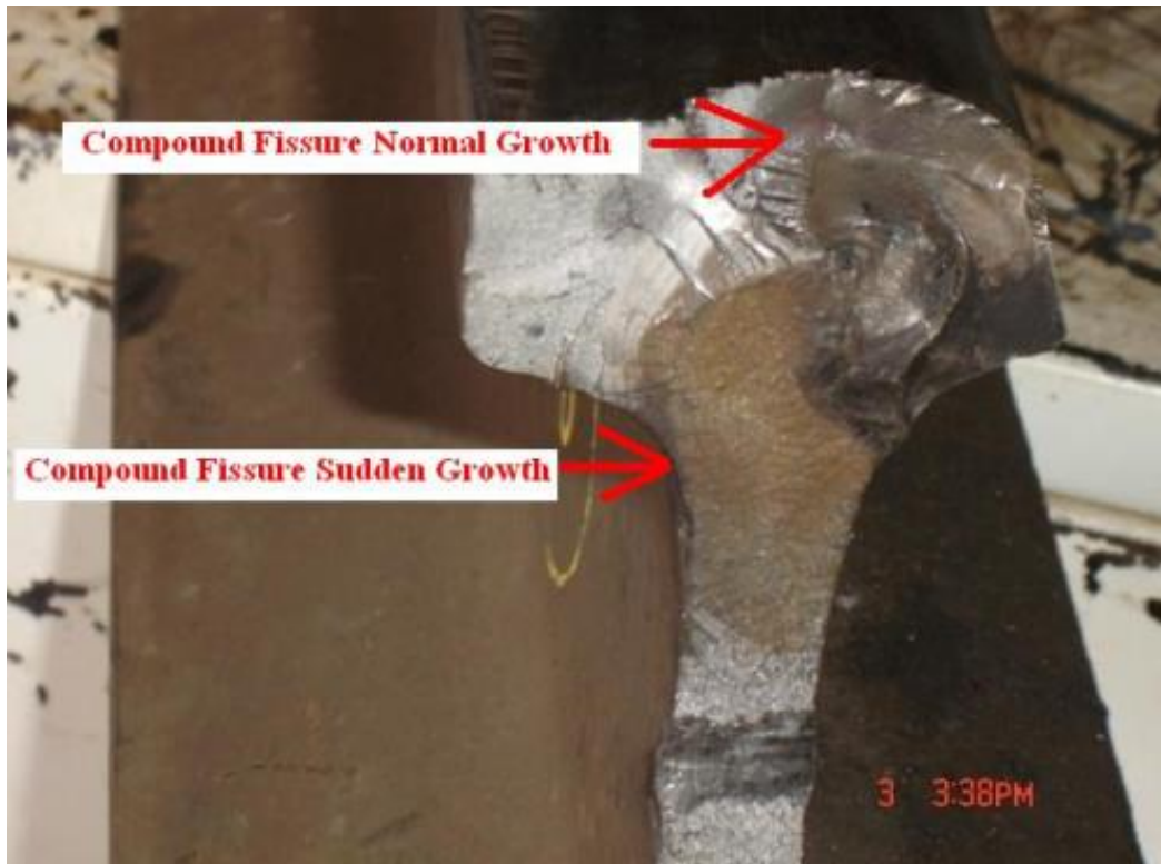
Figure 4-4: Compound fissure defect in the rail head (Federal Railroad Administration, 2015).
