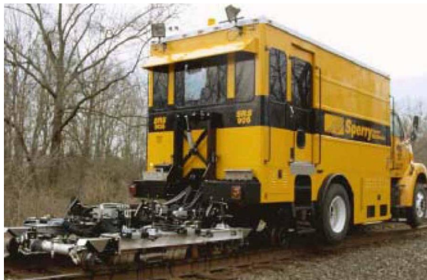
Figure 4-8: Rolling Search Unit used in ultrasonic inspection of rails (Clark, 2004).
