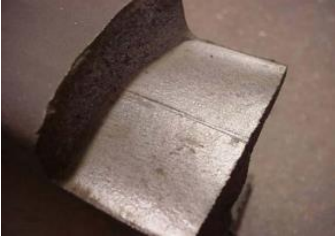
Figure 4-5: Horizontal split head in the rail head from an internal seam defect (Federal Railroad Administration, 2015).
