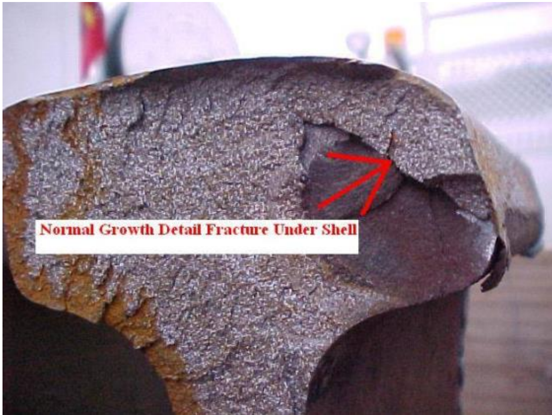
Figure 4-6: Detail fracture defect in the rail head originating from a visible shell defect (Federal Railroad Administration, 2015).
