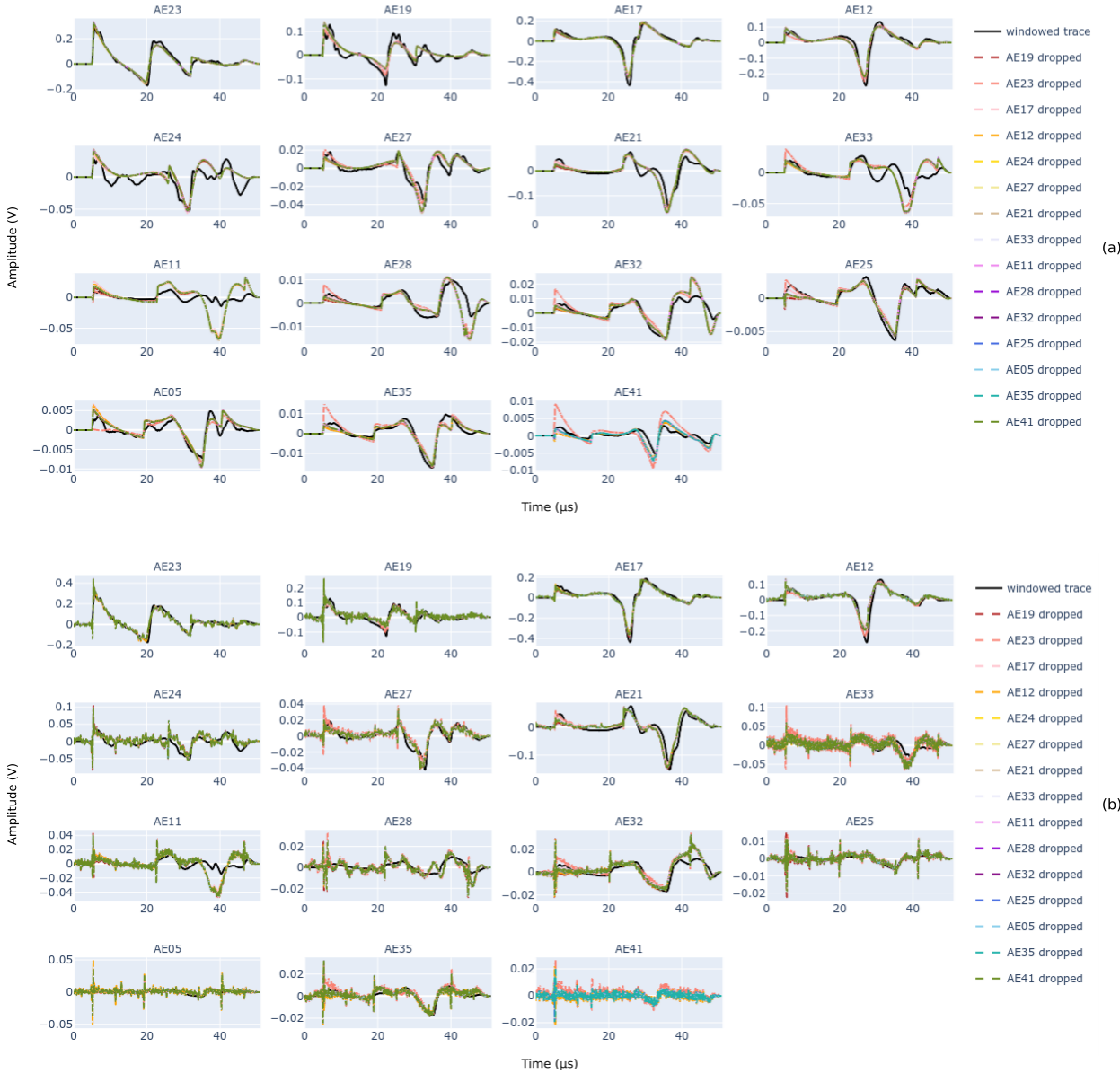
Figure 2.5: Synthetics after force inversion for sample capillary fracture calibration event using (a) scalar calibration and (b) spectral instrument response. The spectral instrument response is applied to the synthetic waveforms by multiplication in the frequency domain rather than dividing it from the experimental records so amplitudes are shown in the recorded units of Volts. The spectral instrument response is not smoothed, resulting in the increased noise shown in (b). The result is shown for the removal of each individual station and little variation is seen, indicating stability in the inversion.
