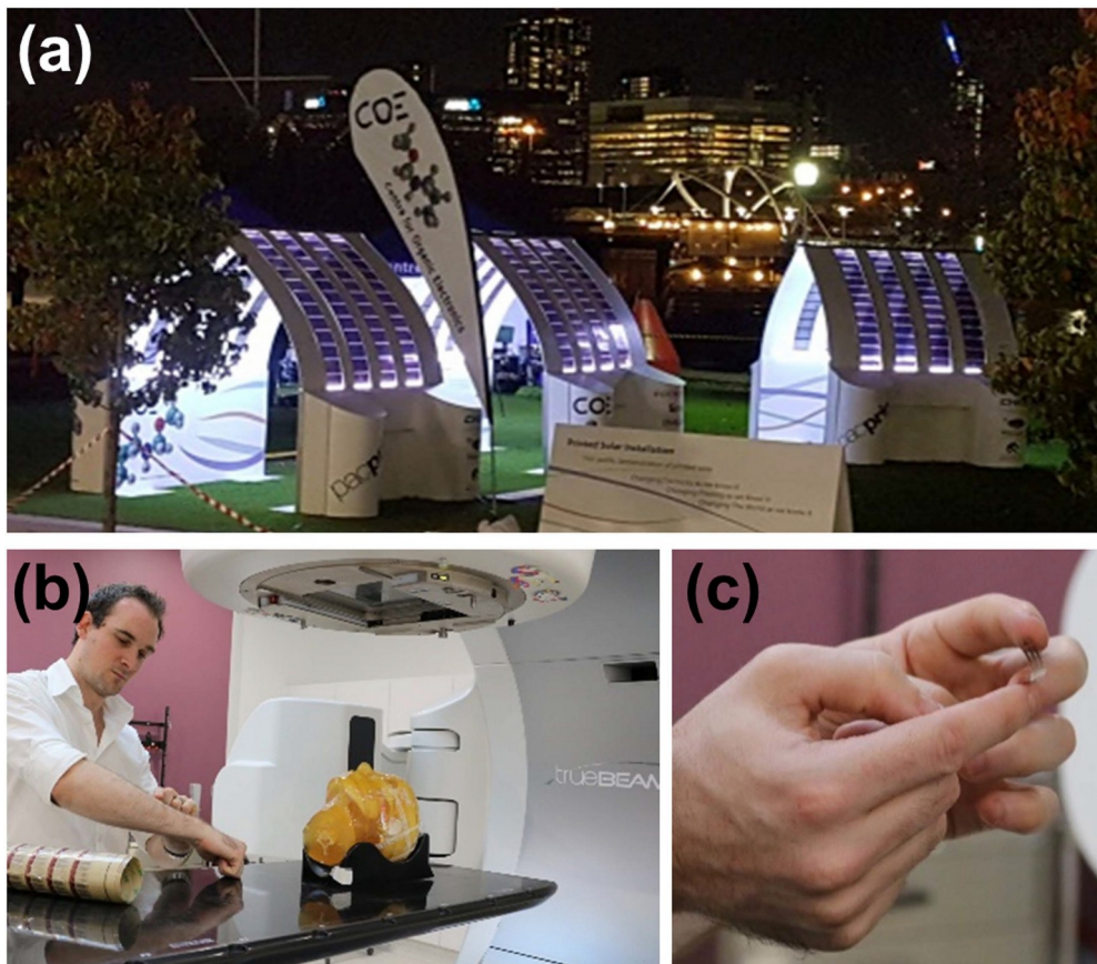
Figure 11. (a) A large area 'solar city' exhibited at Pacprint 2017 in Melbourne (Australia) to demonstrate printed solar cell technology at scale. (b) Radiation detectors printed at scale being investigated with a clinical phantom on a medical linear accelerator, and (c) an expanded view of the flexible printed radiation sensors shown in (b).
