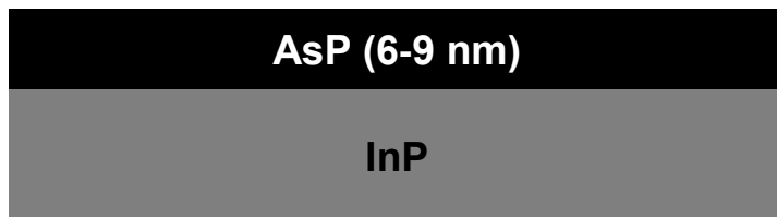
Figure 2.4: Schematic of AsP films grown on InP. The thickness was characterized by x-ray reflectivity. Wafer was directly loaded into diffractometer without dicing for XRR measurements.
