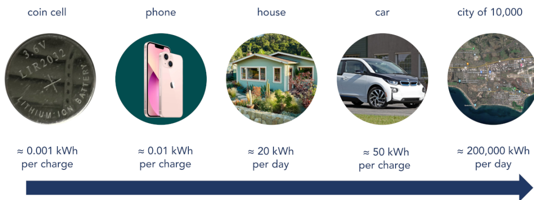
Figure 1.3: A schematic illustrating a range of energy requirements for \text{Li}^+ -ion batteries.
