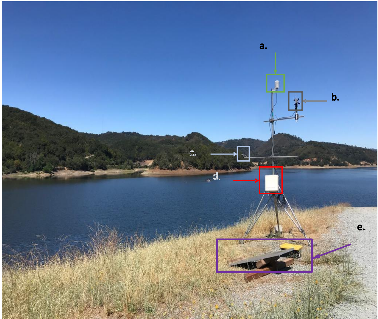
Figure 3.2.3 MET station used throughout the 24-hour studies on Uvas Reservoir. The tower was attached with (a) an air temperature/relative humidity sensor, (b) a wind monitor, (c) a pyranometer, and (d) a Campbell Scientific measurement and data logger CR1000X with a barometer logger inside (e). The station was powered by two 12V Power PS Sonic rechargeable batteries and a 100-watt solar panel.
