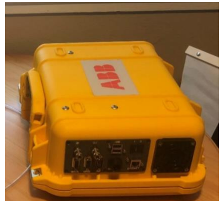
Figure 3.2.2 The LGR gas analyzer that we used for measuring the diffusive flux sample for the study.
